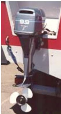
A common problem occurs with kicker outboards that are not electric start. Unless this motor is bonded (connected) to the ground part of the boat, the zinc on the kicker will create a strong positive field around the boat ("hot boat"). This can severely impact your fishing results. Run a ground wire from the kicker to your main engine ground or some other ground point on the boat.
