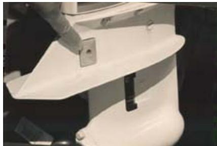
*Most outboard motors have a small zinc anode fastened to the motor shaft. It is very important that this be present and that the motor be bonded to the hull or other metals on the boat.*
