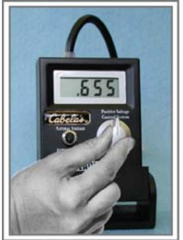
1. Plug in the power to the Black Box. Be sure the Black Box switch is turned to the “off” position (all the way counter clockwise).
