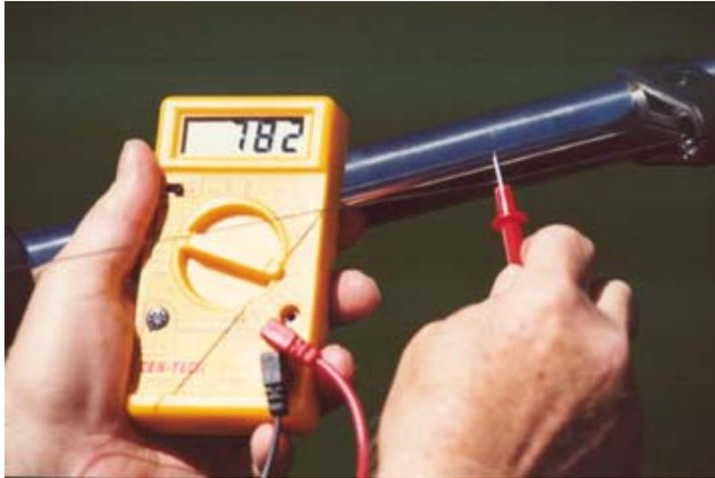
*A voltmeter with a scale of zero to one volt will measure the natural voltage of your wire. Here the natural voltage reading is .782 volts. Note the positive lead is touching the downrigger wire. The negative lead is connected to the engine or the negative pole on the boat battery.*
