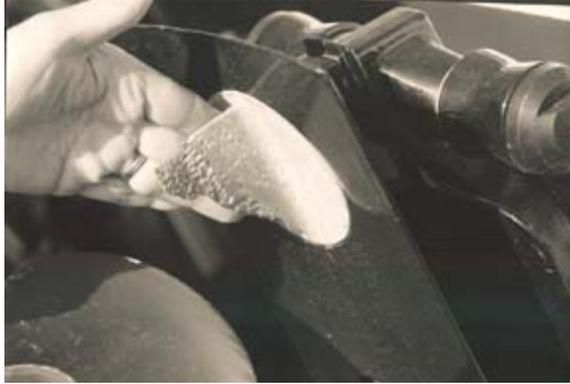
*Zinc anodes are installed on outdrives or motor shafts to protect from electrolytic corrosion. Note the heavily corroded condition of this zinc. When the zinc is more than 50% corroded, it should be replaced.*
